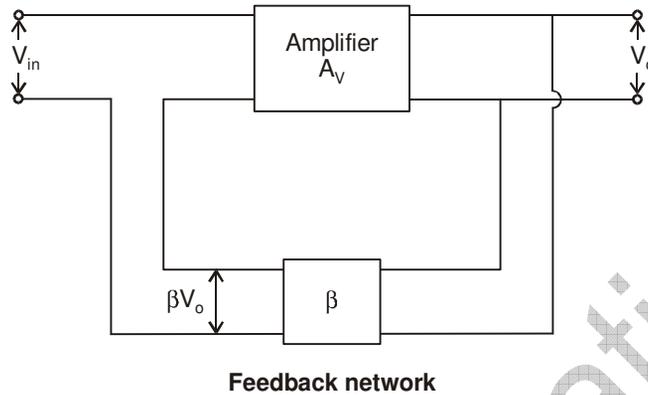
**Figure 2.3: Voltage series feedback connection**
