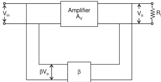
**Figure 2.5: Voltage shunt feedback connection**
