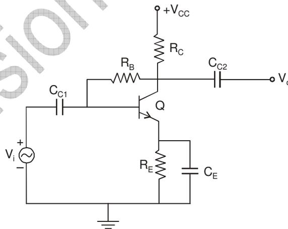
**Figure 2.6: Collector feedback biased common emitter amplifier**
